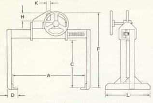
DOWNS Adjustable Pallet Lifting Tongs add extra versatility to the handling of pallets. Adjustable Pallet Lifting Tongs are engineered to handle a wide range of pallet widths using a single tong, giving them a distinct advantage over hooks where the sizes of pallets are varied or irregular. Their ability to be adjusted over a wide range also makes them excellent for handling boxes, cartons, lumber, sheets, and billets. Low headroom design and narrow aisle back-
