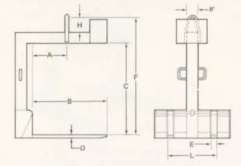
DOWNS Adjustable Fork Pallet Hook allows the forks to be adjusted for unusual or special pallet configurations. The fork carriage of the adjustable pallet hook is similar to that of a standard lift truck. The forks have infinite adjustment over the range of the carriage and are easily moved without the aid of tools of any kind. While under load, the forks are held in place by the weight of the load.
