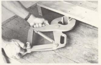
grab any standard  $2 \times 4$  or  $4 \times 4$  pallet stringer or block. Simply attach the *PAL-A-TONG* to any fork truck or winch and pull. A special spring has been provided to hold the tong in place, even when the towline is slack, for easy one man operation.
